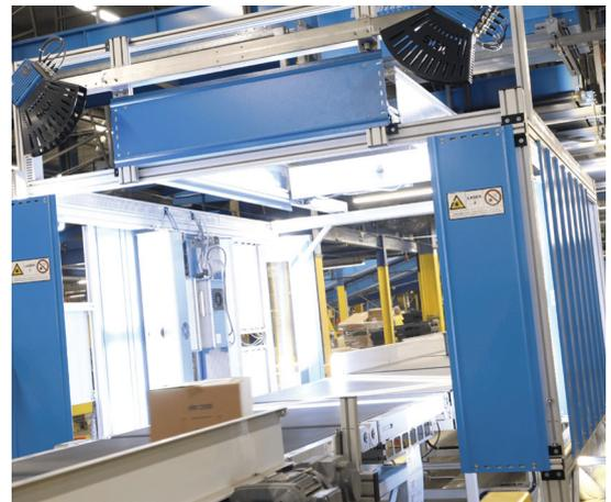
The system, created by Yodel's engineers in response to needs of the booming online retail sector, is capable of processing up to 2,900 one-metre-long items per hour and will work alongside the larger fully automated sort at Shaw. Merlin2 is capable of handling items up to 1.8m long and 0.9m wide and will significantly increase the speed and efficiency of the 'out of gauge' parcel sorting process.
