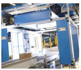
The system, created by Yodel's engineers in response to needs of the booming online retail sector, is capable of processing up to 2,900 one-metre-long items per hour and will work alongside the larger fully automated sort at Shaw. Merlin2 is capable of handling items up to 1.8m long and 0.9m wide and will significantly increase the speed and efficiency of the 'out of gauge' parcel sorting process.
