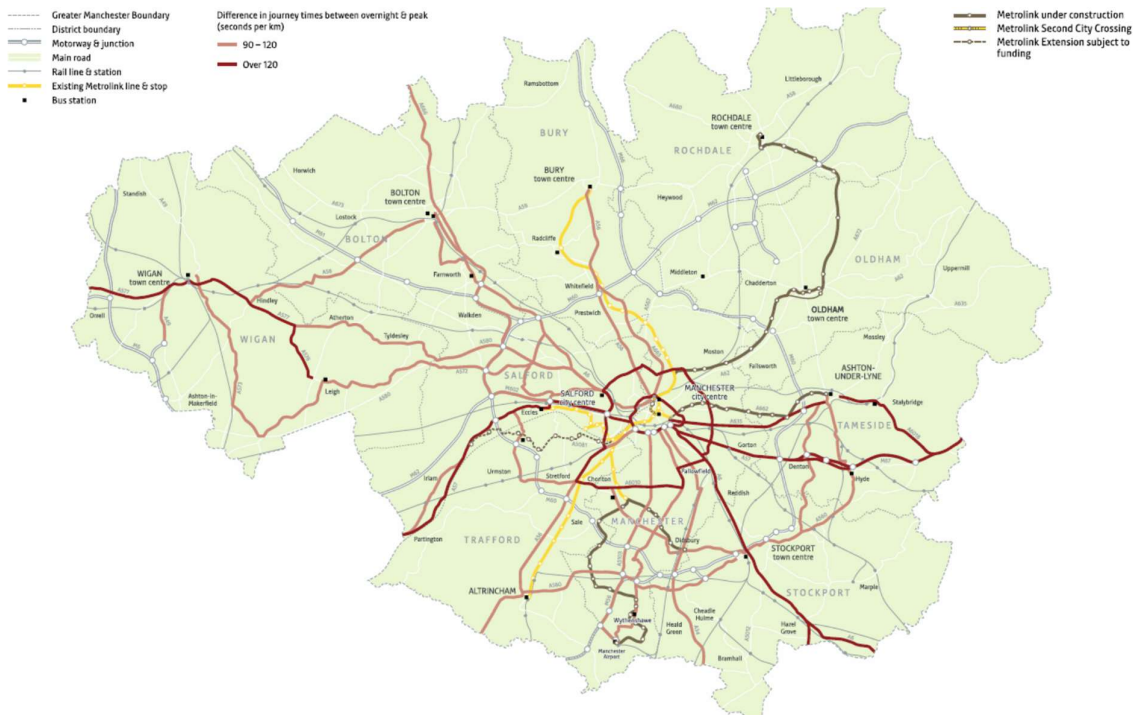
Figure 2-1 Areas of highway congestion across GM
