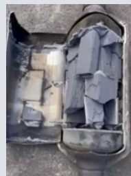
Left to right: legitimate converter core, expanding foam filled and cheaper ceramic replacement.
